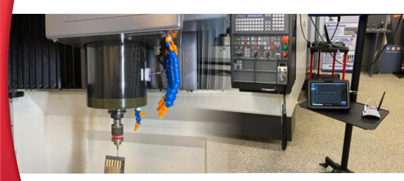
GTI has created a turnkey spindle monitoring system to protect CNC spindles from running unbalanced tools, aggressive cuts, and crashes. This system is constantly monitoring the spindle and has a diagnostic mode for general spindle health including bearing wear.
